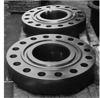
ABOVE: Studding outlets with RTJ facing. BELOW: Blind Bottom stub for economical hydrotesting (eliminates the welding of plugs or blinds).
