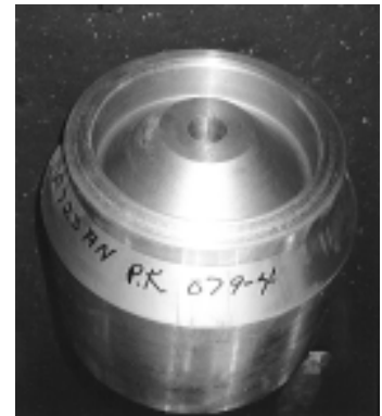
ABOVE: Studding outlets with RTJ facing. BELOW: Blind Bottom stub for economical hydrotesting (eliminates the welding of plugs or blinds).
